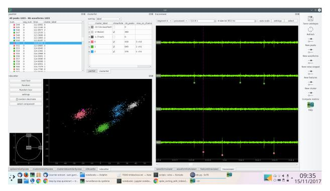
On the right toolbar you can manually re-run some sub steps of the previous chain: detect peak, extract waveforms, extract noise snippets, extract features, cluster.
